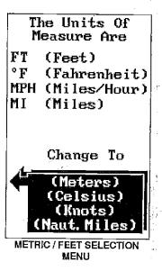
To change the units of measure, first press the MENU key, then press the key adjacent to the "More" label two times. Next, press the key adjacent to the "SELECT UNITS OF MEASURE" label. Now press the key adjacent to the "Change To Meters, Celsius, Knots, Naut. Miles" label. The unit of measure will change to the metric equivalent Repeat the same steps to switch the units of measure again.
